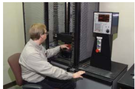
Computer Controlled Spring Testing - Utilizing custom software, spring testers track and verify consistency in spring dimensions and rates.
