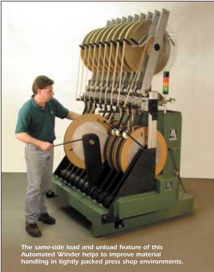
The same-side load and unload feature of this Automated Winder helps to improve material handling in tightly packed press shop environments.
