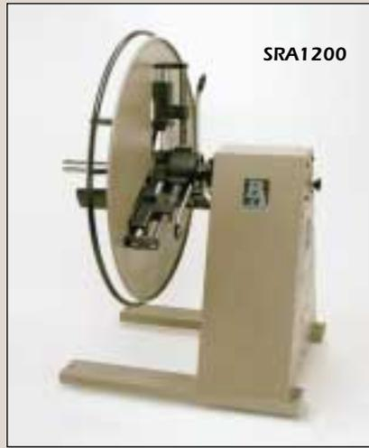
These cabinet reels are recommended for stampers using a variety of applications that require a free loop of material at all times. The efficient DC Drive package ensures that the reel will automatically compensate, without operator adjustments, for the inches of material per minute required for any of your jobs.
