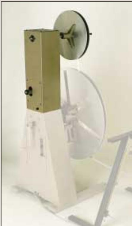
Large reels may be fitted with paper interleaf options. These self-contained units are designed to be mounted on our motorized reels and are available in two basic types.
