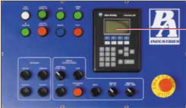
Allen Bradley Controls with self-diagnostic error message display
