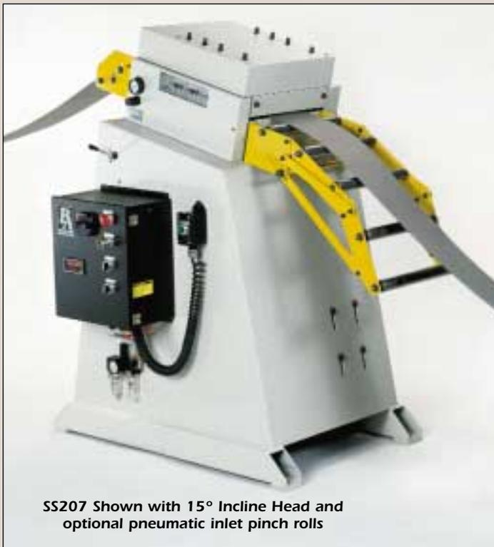
SS207 Shown with 15° Incline Head and optional pneumatic inlet pinch rolls
