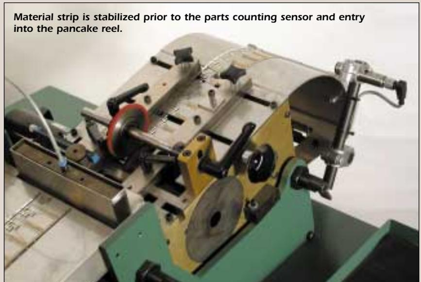
Material strip is stabilized prior to the parts counting sensor and entry into the pancake reel.
