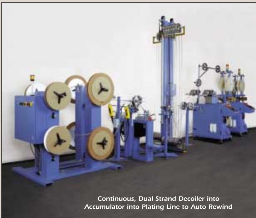
Continuous, Dual Strand Decoiler into Accumulator into Plating Line to Auto Rewind
