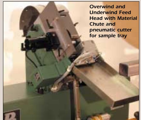
Overwind and Underwind Feed Head with Material Chute and pneumatic cutter for sample tray
