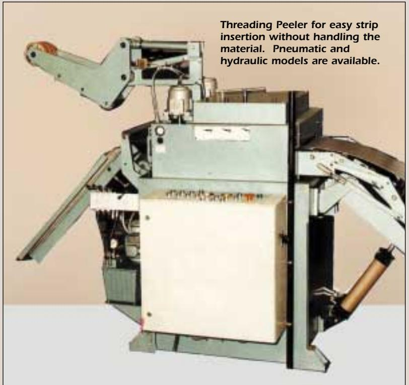
**Threading Peeler for easy strip insertion without handling the material. Pneumatic and hydraulic models are available.**
