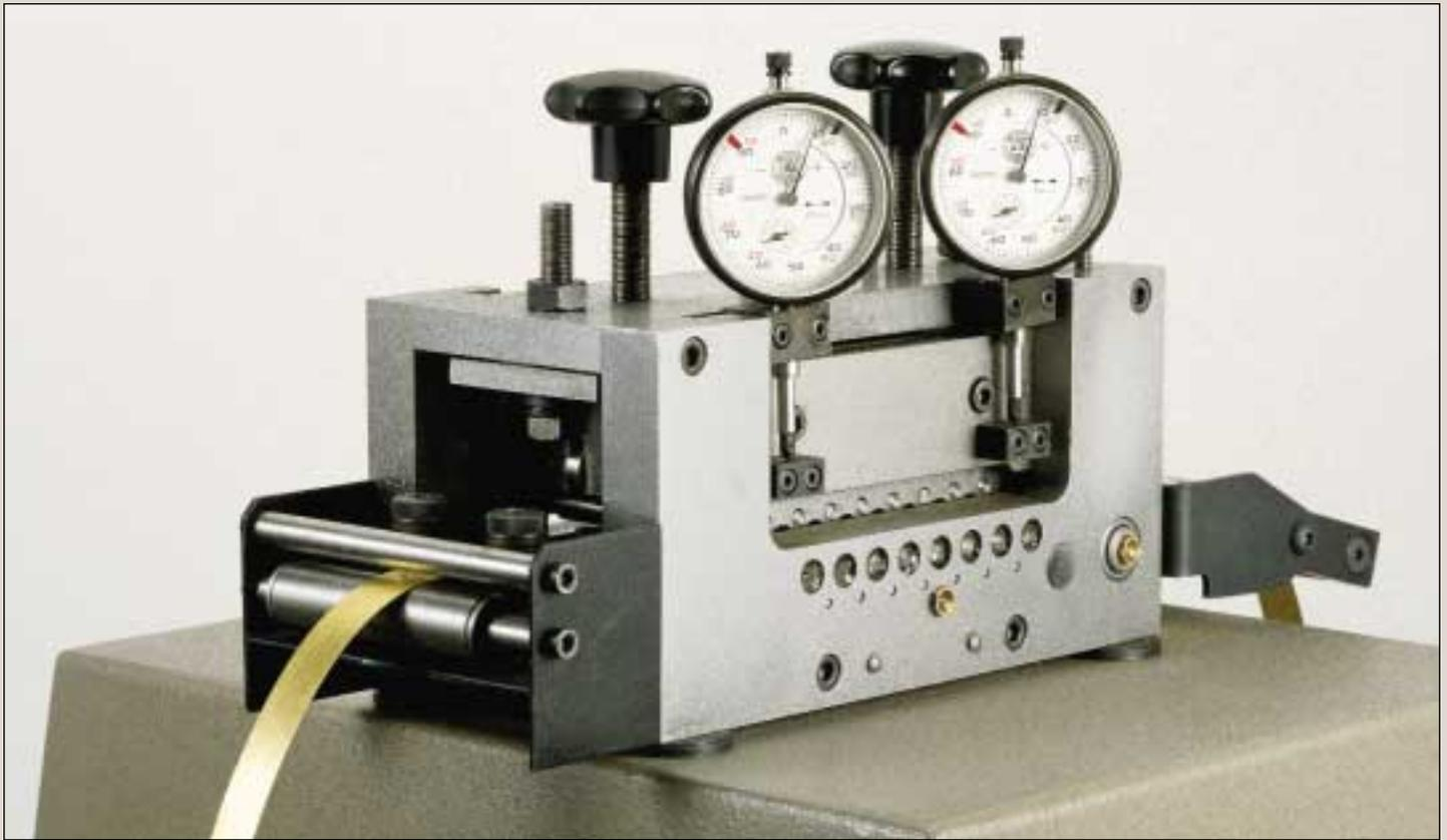
The P/A Ultra Precision Stock Straightener was designed with the electronics stamper in mind, especially those using exotic coppers or clad materials in their operations. A very unique design employs seventeen straightening rolls which are backed up by roller bearings in a precision machined steel body.
