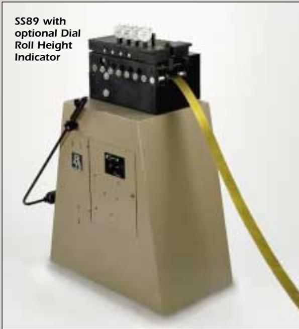
The advantages of these straighteners are immediately obvious. The Flip Top makes strip loading easy. Simply swing open the head, feed in the strip, close and tighten. Single-point adjustment for each roll ensures a precise setting and eliminates the cambering often caused by nonparallel rolls.
