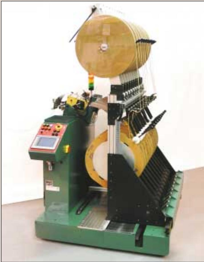
Lower your Man-to-Machine Ratios or run unattended with up to 10 reels of Automated Winding.
