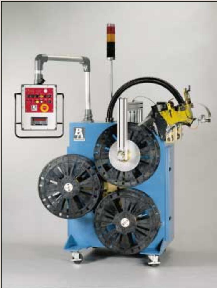
The LW 24-3 Traverse Layer Winder is a 24-inch, 3 station, automatic material winder capable of continuous operation when assisted by an operator.
