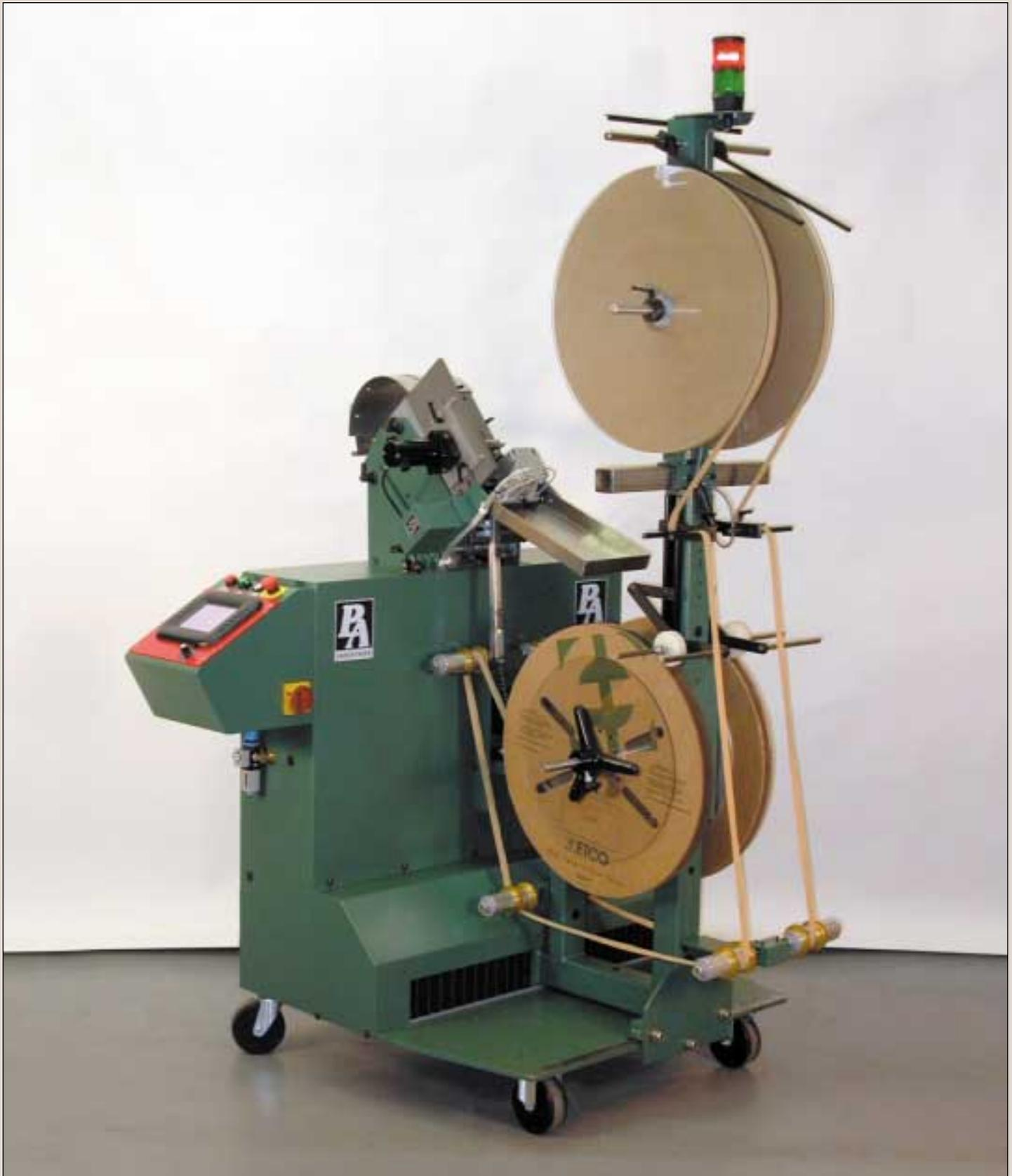
Increased productivity is the motivation behind the introduction of entry-level automation. These compact, high-speed units perform automated reel changes based on a pre-programmed number of parts per pancake reel without stopping the press. This makes them ideally
