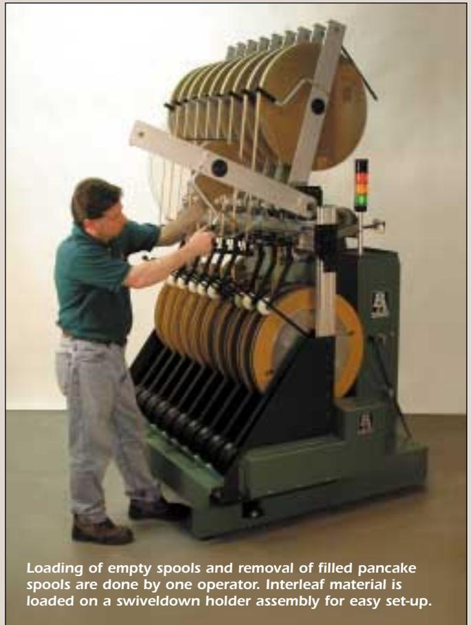
Loading of empty spools and removal of filled pancake spools are done by one operator. Interleaf material is loaded on a swiveldown holder assembly for easy set-up.
