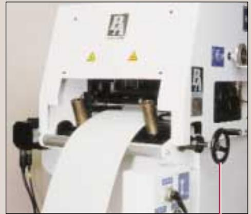
Handwheel, self-centering material roller, edge guides and separate stock position adjustment
