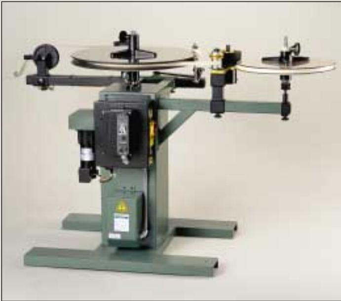
Our Horizontal Winder Reel was designed for winding processed material in the horizontal mode. Horizontal winding is desirable when winding terminal strips with a carrier strip located downward for smooth winding of the strip onto the spool. A reel is equipped with paper interleaf payoff and a variable speed infrared loop control. Optional magnetic paper tension brake mat be provided for precision control of paper tension.
