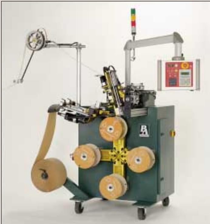
The LW 15-4P is a fully automatic traverse winder equipped with a universal material feeding and guiding head. The winder automatically inserts the strip into the empty spool and fills the spool until the preset number of terminals is reached.
