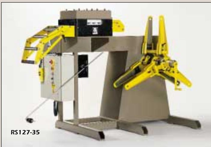
When floor space is at a premium, consider this Space Saver design by the innovative P/A engineering team. The Stock Reel is equipped with an adjustable caliper disc brake to provide the right amount of back tension. The DC drive Stock Straightener is offset for easy loading. The loop-sensing arm automatically adjusts material payout speed to press requirements. These units are equipped with entrance cascade and exit pinch rolls. Specify left-to-right or right-to-left stock travel.
