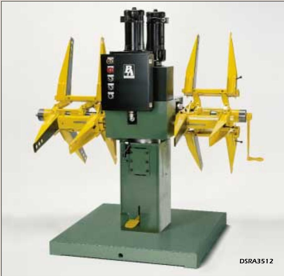
These Dual Reels use the same rugged construction as that of the Single Reels. The motorized versions have two proportional speed DC or AC motors, one for each spindle. Each drive motor uses a gear reducer with torque limiter for additional gearbox protection.
